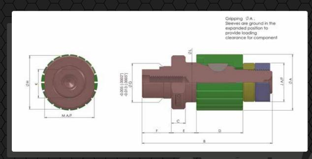
The nut operated between-centres expanding mandrel is generally mounted between 60 degree centres, and can be driven from the drive flat with a carrier or drive plate. It is possible to attach a simple component end locator, if required, at diameter L.
