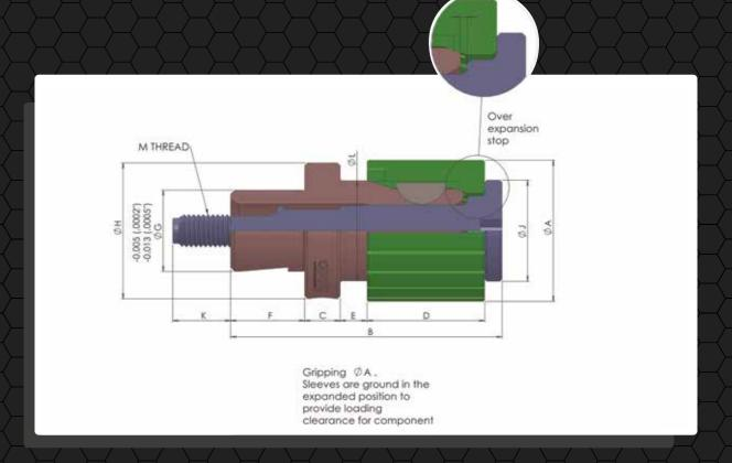
The spigot drawbar operated expanding mandrel can be used on any machine with drawbar facilities, for general turning and grinding operations.
