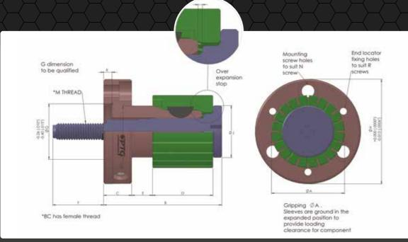
The faceplate drawbar operated expanding mandrel can be used on any machine with drawbar facilities, for general turning and grinding operations.
