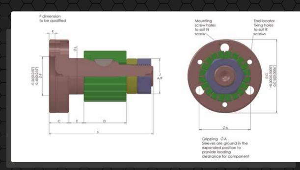
The face-plate nut operated expanding mandrel can be used on any machine with no drawbar facility, for general turning and grinding operations. These are a popular choice for milling fixture locators.
